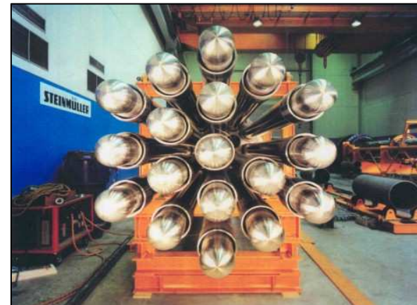
10 MW steam CH 4 reformer mock-up for nuclear application
