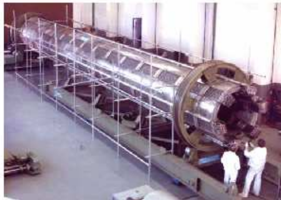
10 MW mock-up of a He-He heat exchanger
