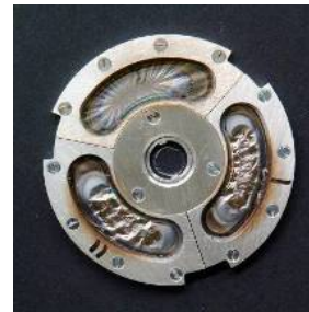
targets mounted on the wheel for TASCA project Transactinide Separator and Chemistry Apparatus
