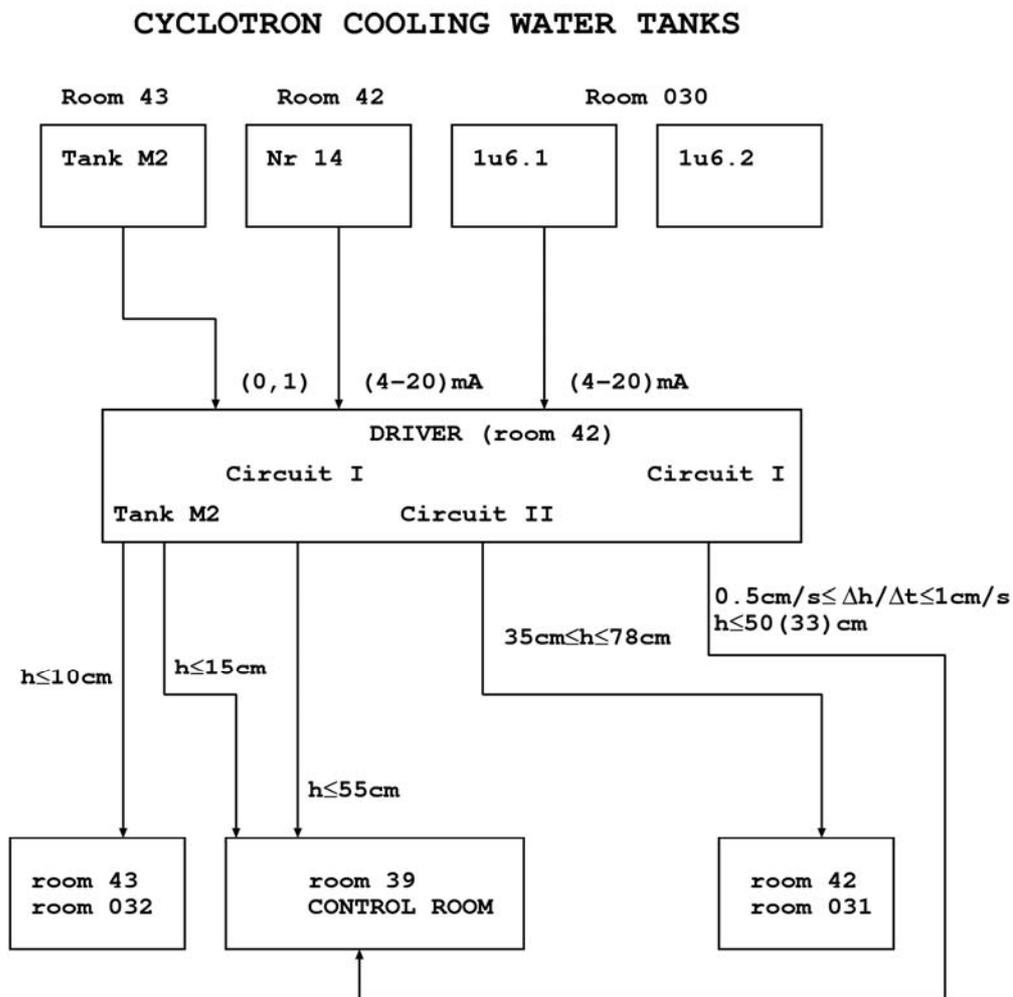
**Fig.1.** Block scheme of the cooling circuit.
