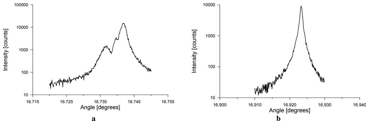
Figure 2. Rocking curves recorded in (511) asymmetric reflection of 0.115 nm radiation with small point probe beam  $50 \times 100 \mu\text{m}^2$  from samples 1 (a) and 3 (b).
