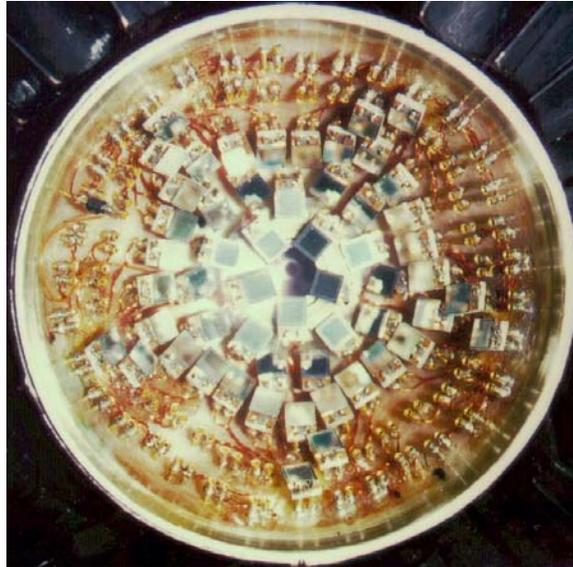
**Fig 1.** The particle detector chamber showing the PIN – diodes distribution (beam dump side view).
