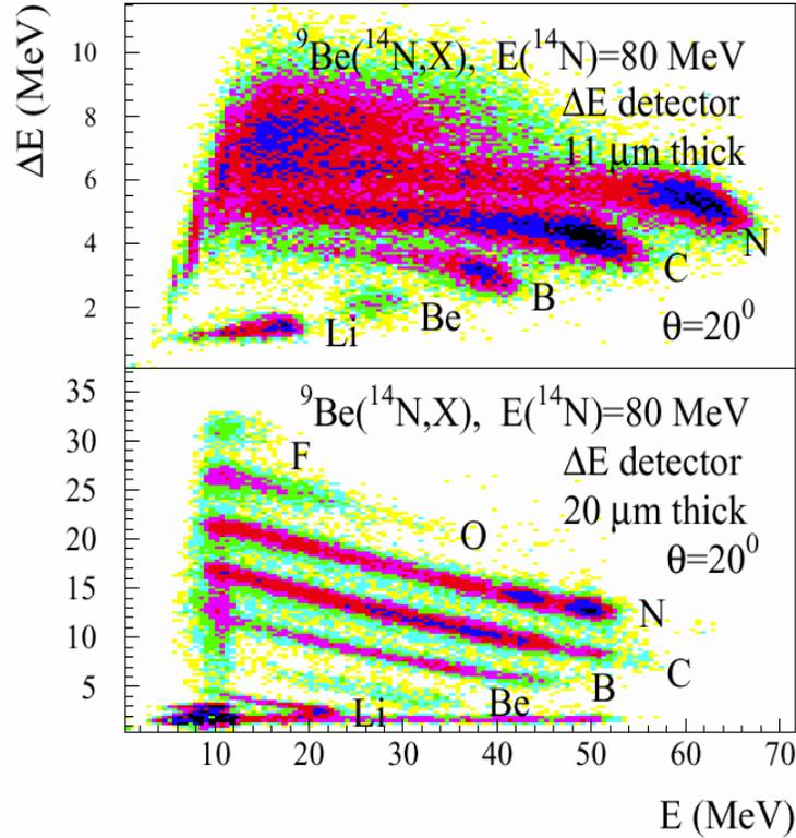
**Fig. 2.**  $\Delta E$ -E scatter plots obtained after irradiation of the monolithic telescopes with  $^{12}\text{C}(^{14}\text{N}, X)$  reaction products. The upper frame - results for the monolithic telescope with 11  $\mu\text{m}$  thick  $\Delta E$  detector, the lower frame - results for the monolithic E- $\Delta E$  telescope with 20  $\mu\text{m}$   $\Delta E$  detector. In both cases the pulse shape analysis technique was applied.
