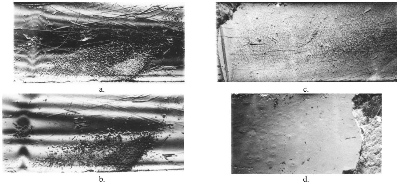
Figure 1. Monochromatic beam topographs from: (a) and (b) - sample 1 taken for different angular positions, (c) - sample 2, and (d) - sample 4.
