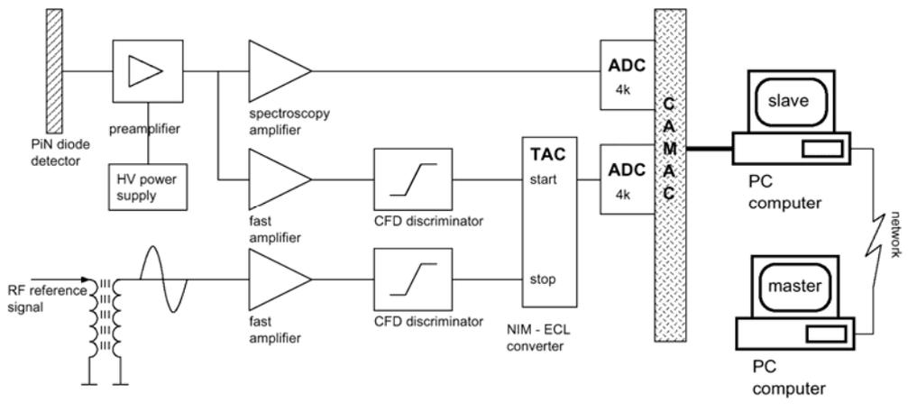
**Fig. 2.** Electronics for the beam diagnostics system
