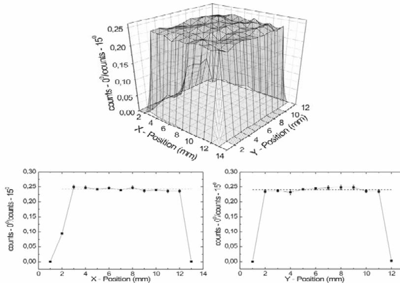
**Fig. 2.** Measured two dimensional plot of the  $^{12}\text{C}$  ions intensity scattered over the  $1 \times 1 \text{ cm}^2$  exit window at the cell container position normalized to the intensity of the elastically scattered ions at the  $15^\circ$  silicon detector (a) and the profiles in x- (b) and y-direction (c).
