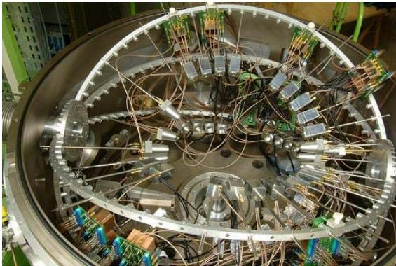
Fig.1. ICARE detectors inside the chamber
