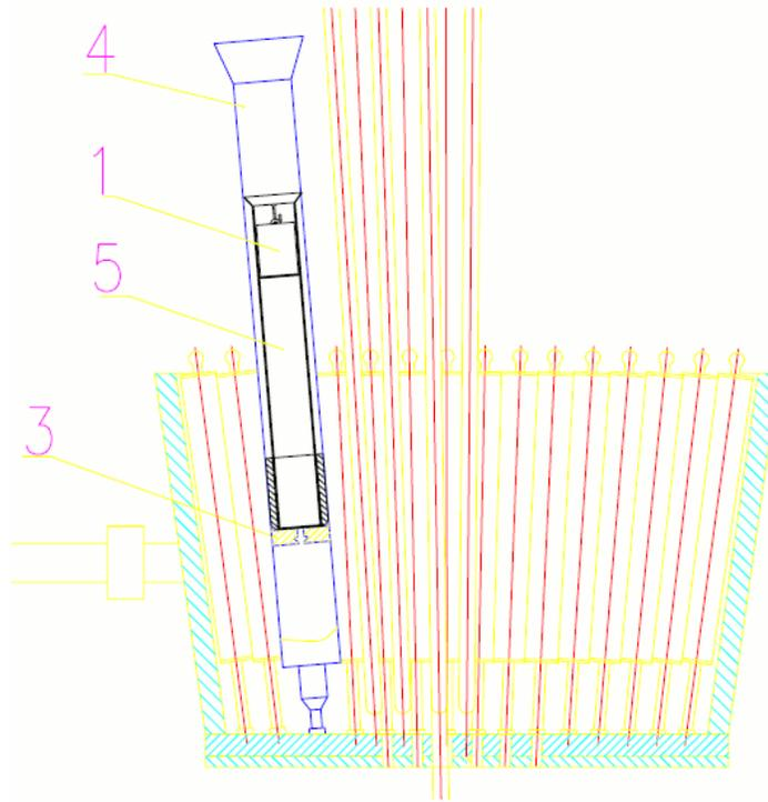
**Figure 2:** “Virtual” V1 vertical channel of reactor Maria with thermal neutron flux intensity about  $10^{12}$  neutrons/s/cm<sup>2</sup>. 1 – container for silicon wafers, 3 – graphite block, 4 – basket surrounding the channel, 5 – V1 channel
