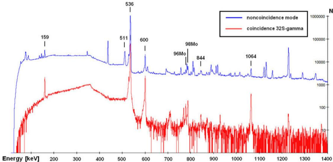
**Figure 1:** The particle-gamma coincidence spectrum (red) compared to the non-coincidence spectrum (blue) collected by a single HPGe detector.
