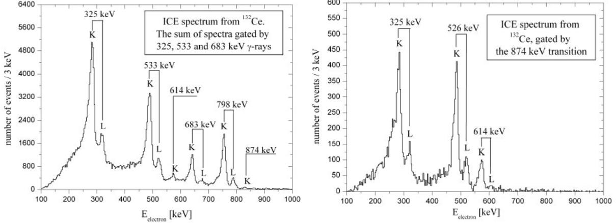
**Figure 2:** *Left panel:* Summed electron spectrum observed in coincidence with the 325, 533 and 683 keV gamma-ray transitions. *Right panel:* Electron spectrum observed in coincidence with the 874 keV  $\gamma$ -ray transition.
