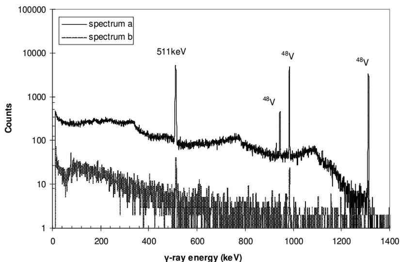
**Figure 2:** Gamma-ray spectra (spectra a and b) collected after centrifugation of the colloidal TiO<sub>2</sub> solution. Spectrum (a) corresponds to the TiO<sub>2</sub> pellet while the spectrum (b) to the suspension solution, which shows much lower activity of <sup>48</sup>V with respect to spectrum (a).
