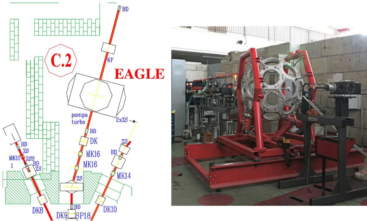
**Figure 1:** *Left:* Present arrangement of the C2 beamline. *Right:* C2 beamline and EAGLE supporting structure – status at the beginning of May 2009.
