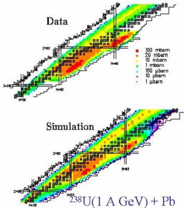
**Figure 1:** Experimental and calculated (ABRABLA code) nuclide production cross-sections.
