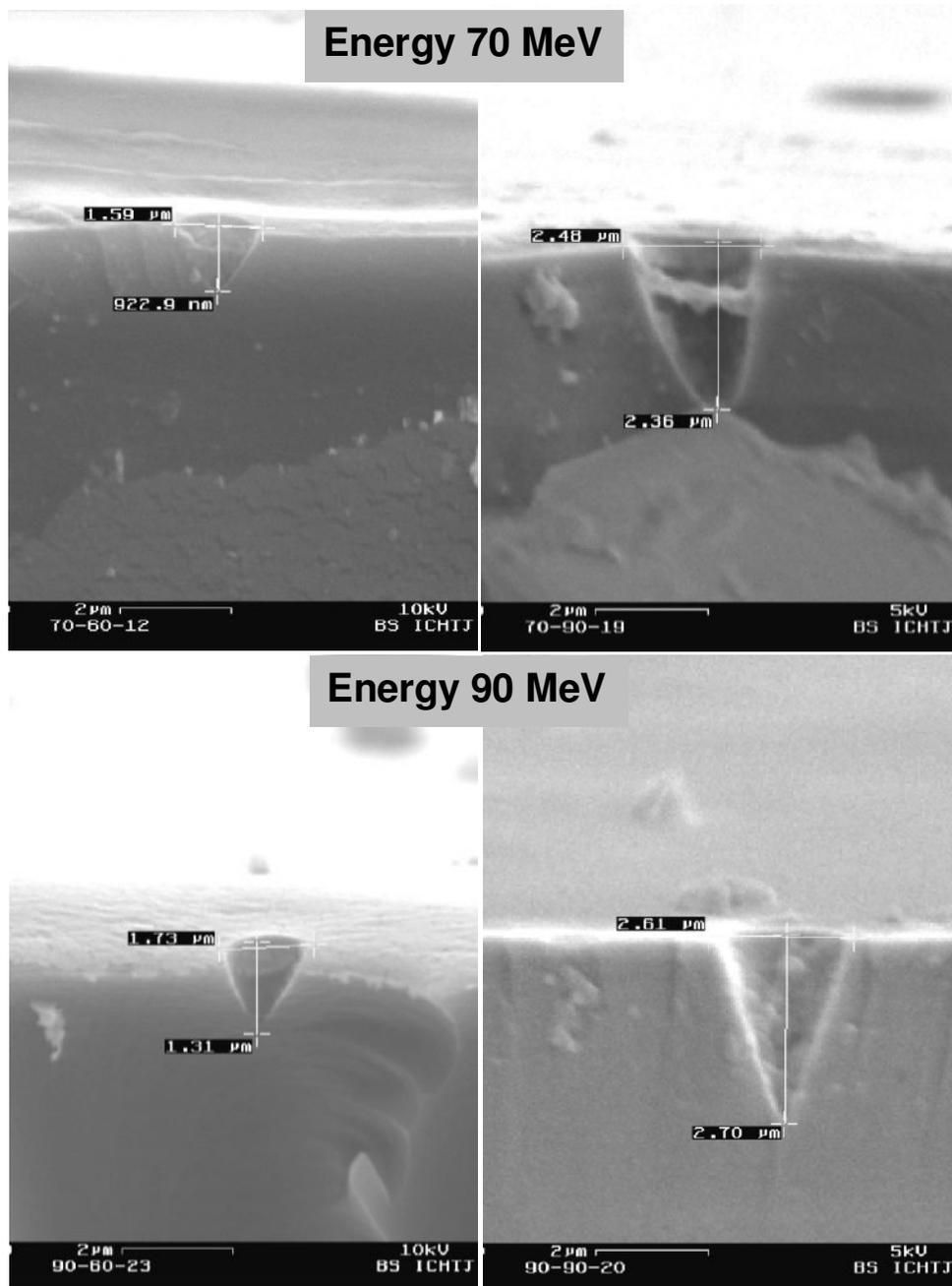
**Figure 3:** Shape evolution of tracks produced by C ions of two different energies in the PM-355 detector, as a function of etching time. The tracks on the left side were etched for one hour and the ones on the right for 1.5 h.
