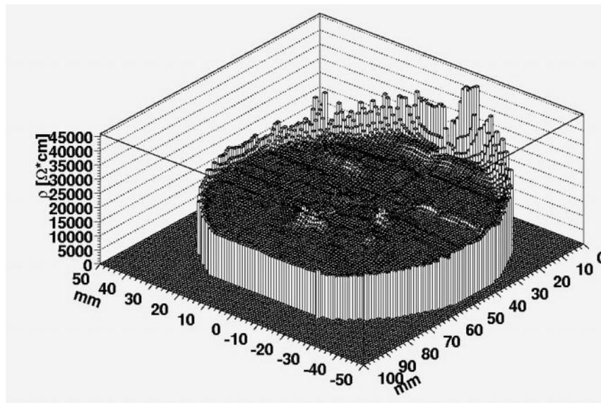
**Figure 1:** Four inch wafer resistivity as a function of position.
