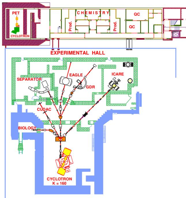
**Figure 1:** The location of the Radiopharmaceuticals Production Centre in the Laboratory building in the basement of 360 m<sup>2</sup> at 6 m depth. The figure shows also the K=160 heavy ion cyclotron, beam lines and presently operating experimental set-ups.
