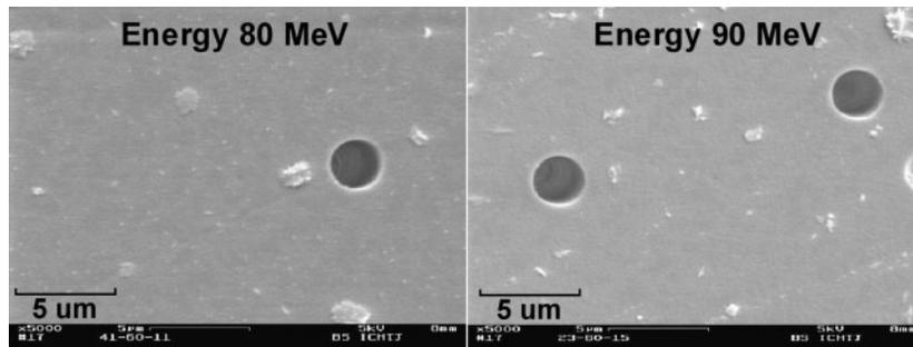
**Figure 2:** Exemplary photos of the craters induced in the PM-355 detector samples irradiated by C-ions of different energies. The samples were etched for one hour.
