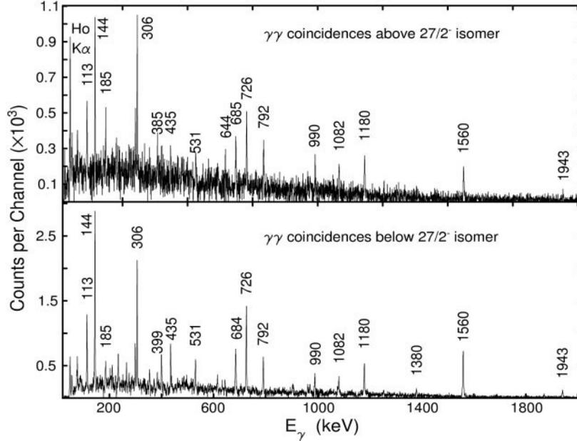
**Figure 2:** *Bottom:*  $\gamma$ -ray sum spectrum gated by the  $\gamma$  rays deexciting the  $27/2^-$ , 59 ns isomer in  $^{149}\text{Ho}$  showing also the weakened lines deexciting levels above the isomer. *Top:*  $\gamma$ -ray sum spectrum gated by the  $\gamma$  rays feeding the 59 ns isomer showing the weakened lines deexciting levels below the isomer.
