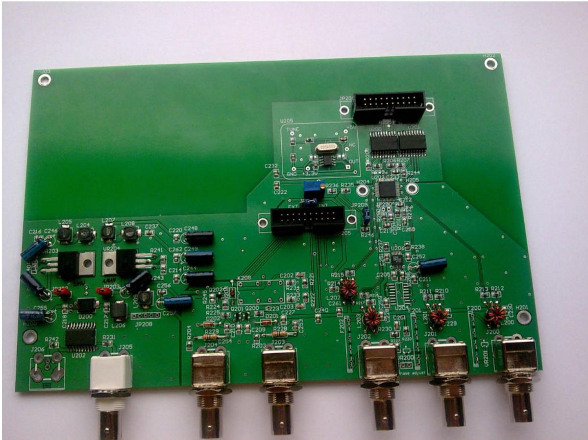
The board was designed, assembled, and first electrical tests were made. The next test will be the DDS functional test using direct computer control via parallel interface from the computer side. Then the “digital board” will be designed, assembled and the microcontroller program will be written.
