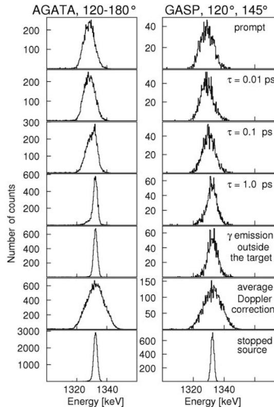
**Figure 1:** Simulated shapes of transitions registered in AGATA and GASP, for different life times of the state emitting a 1.3 MeV  $\gamma$  ray.
