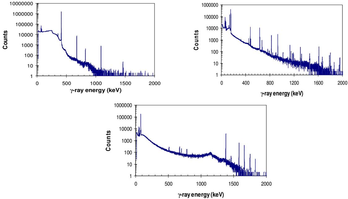
**Figure 2:** Gamma-ray spectra of activated pure Au, Re and Ho foils irradiated in the neutron activator. The  $\gamma$ -ray peaks of  $^{198\text{g}}\text{Au}$  (top left),  $^{198\text{g}}\text{Re} / ^{196\text{g}}\text{Re}$  (top right) and  $^{166\text{g}}\text{Ho}$  (bottom panel) are all well resolved.
