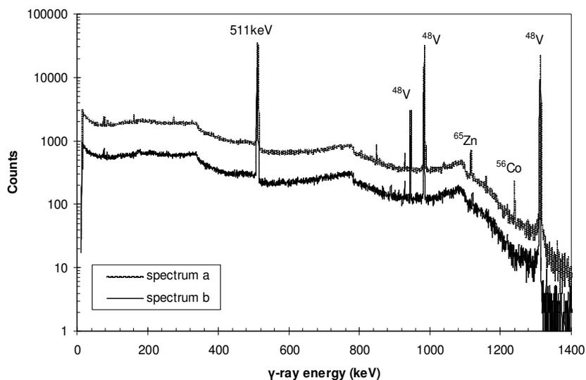
**Figure 1:** Gamma-ray spectra of the proton-irradiated TiO<sub>2</sub> powder. Spectrum (a) refers to the irradiated TiO<sub>2</sub> powder contained in an Al capsule while spectrum (b) corresponds to the TiO<sub>2</sub> powder removed from its capsule. The  $\gamma$ -ray peaks of <sup>48</sup>V are well resolved in both spectra. The  $\gamma$ -ray peaks of <sup>56</sup>Co, <sup>65</sup>Zn are due to the impurities of the Al capsule (spectrum a) which were activated.
