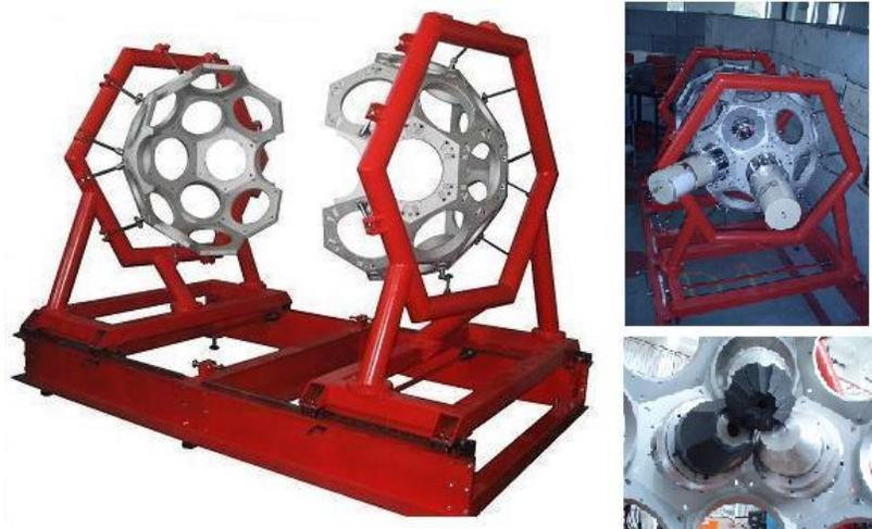
**Figure 1:** Supporting structure of the EAGLE array (left) with three different kinds of detectors mounted (right).
