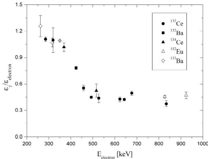
**Figure 1:** The experimentally determined efficiency curve ( $\varepsilon_\gamma/\varepsilon_{\text{electron}}$ ).
