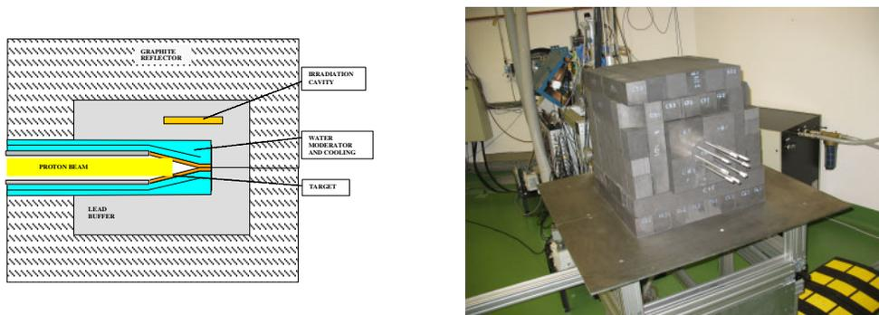
**Figure 1:** Left: Sketch of the neutron activator. Right: Photograph of the neutron activator installed in a beam line of the JRC cyclotron.
