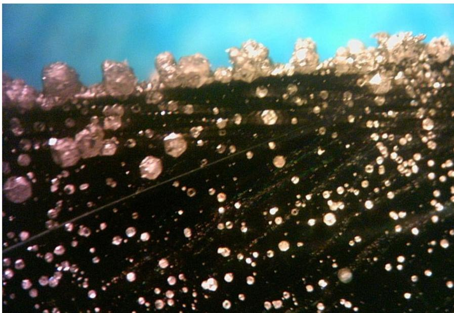
**Figure 1:** Diamonds grown by MW CVD epitaxial process on a silicon substrate.
