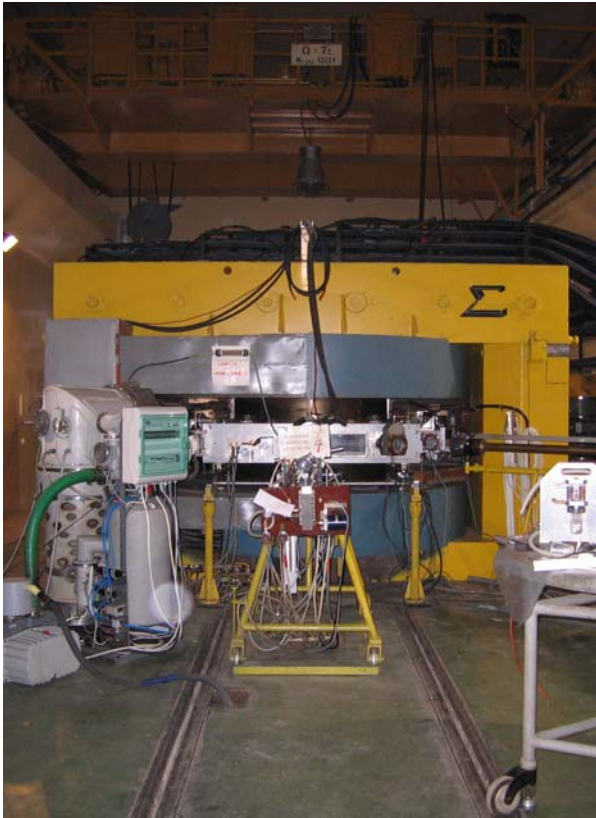
Fig. 4. AIC-144, K=60 light particles cyclotron operating at Institute of Nuclear Physics in Kraków.
