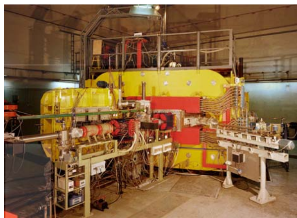
Fig. 2. The K_{max}=160 heavy ion cyclotron of the Warsaw University.
