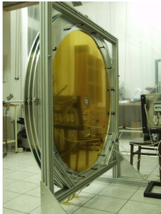
Fig. 1. Prototype drift chamber for PANDA. The chamber contains four detection planes with square 1cm x 1cm cells. The central opening is foreseen for the beam pipe.
