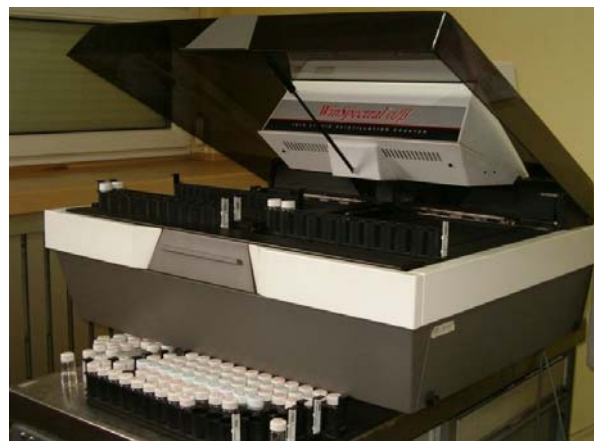
Fig. 1. Liquid Scintillation Counter 1414 \alpha/\beta from Wallac at the Laboratory of Low Activities.
