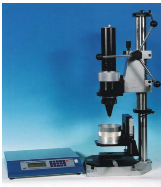
Fig. 6. The dose-rate activity gauge MAD-2000 for measurements of the dose rate and activity of ^{106}\text{Ru} and ^{125}\text{I} brachytherapy applicators for eye cancer radiotherapy, developed at ICHTJ.
